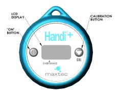
**LCD Display:** A 3-digit display provides a direct readout of oxygen concentration in the range of 0 - 100%. The display is blank when the Handi®+ enters its Sleep (power off) mode. The Handi®+ will automatically enter the Sleep mode after approximately 1.3 minutes from the last time the ON button was pressed.
